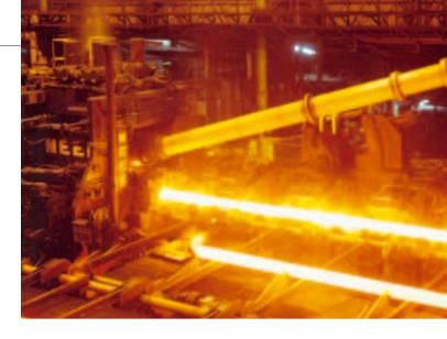
We produce our steel through the electric arc furnace route. The raw material mix is chosen and prepared carefully to ensure the highest standards of cleanliness. All heats are ladle refined and vacuum degassed before continuous casting and rolling. Right through the production process, we maintain full traceability of the material and a record of the tightly controlled process parameters. This ultra-clean steel forms the starting point for the manufacture of our fuses.
